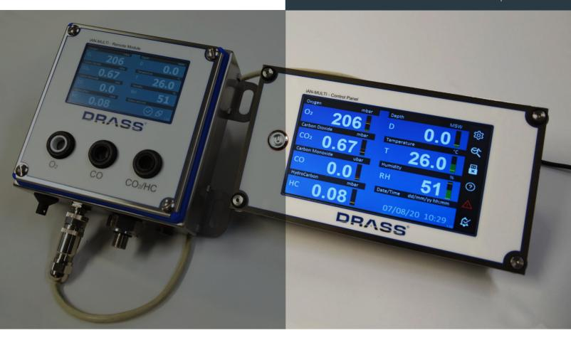
The Control Panel can be interfaced to external systems using embedded Ethernet and RS485 ports. Each system, composed of a Control Panel and a Remote Box, is individually tested and calibrated before delivery; also, the system comes with required ancillaries to permit calibration on site (calibration gas to be sourced locally).
