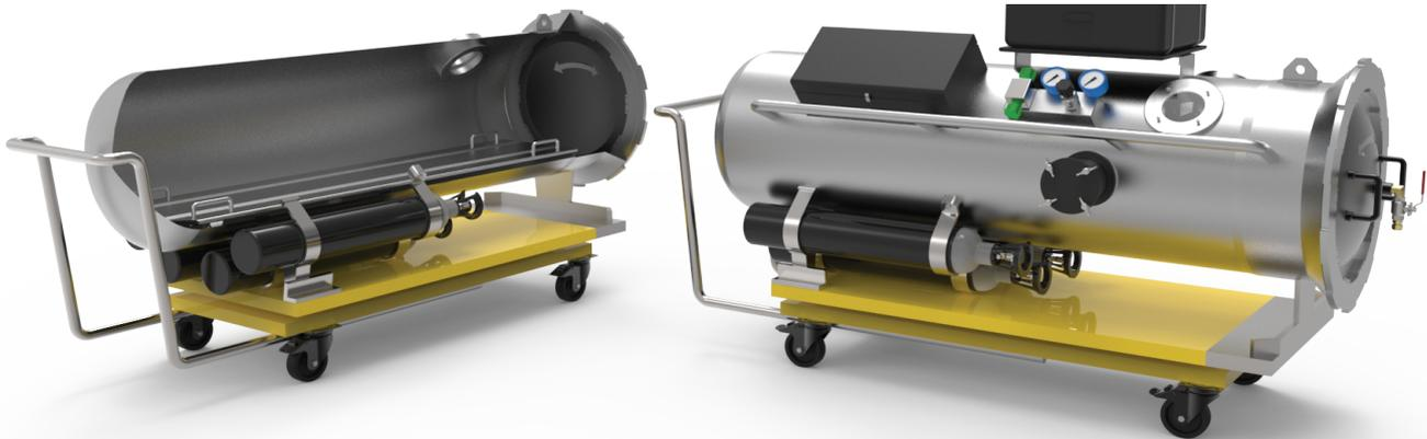
**DRASS DRASSUNO** is a one-man portable hyperbaric chamber for commercial, military, rescue, or scuba diving. Built with an internal diameter of 650 mm, DRASSUNO is designed to support shallow water diving operations in areas, such as onboard vessels, where emergency access to a fixed recompression chamber is not available. DRASSUNO can accommodate and medically treat a diver, permitting an immediate recompression on site at 70 msw in the event of a diving accident.
